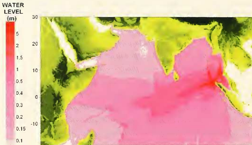
Figure 3. Computer modelling of the 26 December, 2004 tsunami after 900 minutes (courtesy of A. Yalciner, U. Kuran, T. Taymaz) (available at: http://yalciner.ce.metu.edu.tr/sumatra/max-elev-sim-1.jpg ).
